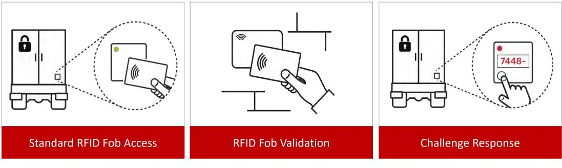
Access to FreightLock is gained via an RFID fob, which can be programmed to access individual vehicles or groups of vehicles. Validate individual fobs to enable to access to your vehicles for a pre defined period of time (i.e 12 hours, 24 hours, 1 week etc), thus offering greater control over the number of access fobs in circulation. A powerful feature that negates the requirement for access keys.
