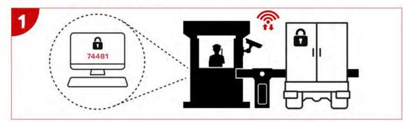
As the vehicle arrives at the gatehouse, the seal data is automatically uploaded to your secure database at www.integritas-secure.net. The current seal number and vehicle details are displayed on a screen in the gatehouse so it can be verified against the delivery manifest.
