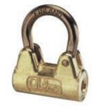
This padlock has a die-cast, compact brass body and is non-sparking as it has no steel parts. Furnished with raised shoulders for added strength and shackle clearance, this general purpose padlock is a cost-effective way of securing boats, bicycles, tool boxes, storage sheds, and power station switches. It also provides a secure method of closure in applications where sparkfree performance is essential. Shackle diameter 7 mm.
