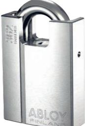
For applications where maximum security is required. Case-hardened steel body with raised shoulders and a top-loaded cylinder provide the highest level of security and protection. Applications include containers, train wagons, trucks, lorries, heavy sliding doors, military applications etc. PL362 is equipped with a case hardened boron steel shackle, diameter 15 mm.
